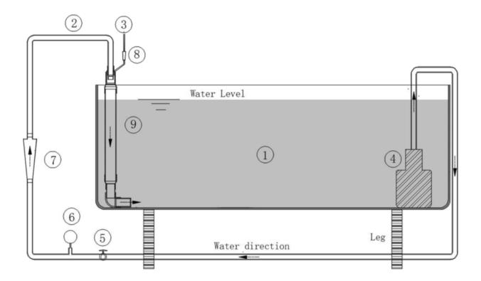
Figure 1:Diagram of the aeration system used in the experiment
